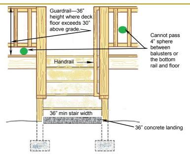
All decks 30" high or more above finished grade, are required to have a guardrail. Note: If you are providing a guardrail were the deck 29" or less the guardrail must meet the same requirements.
