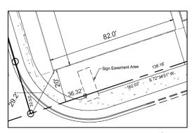
Additionally, as shown on the site plan, the sign easement area appears to encroach into the existing right-of-way of U.S. Hwy. 78 (E. Main Street).
