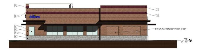
The applicant's letter of intent states that proposed fenestration would be 42.4%. While dimensions are not shown on the submitted building elevation, the site plan identifies the width of the building to be 82 feet. It appears as the proposed blank wall area may be less than 40 feet. A variance may not be required as the applicant has requested.
