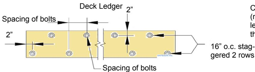
Correct placement of fasteners in deck ledgers (rim joists). Bolts must be placed in the deck ledgers as shown with spacing determined by the below table.
