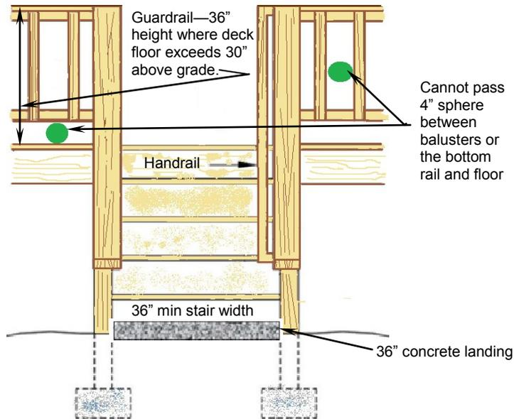
All decks 30" high or more above finished grade, are required to have a guardrail. Note: If you are providing a guardrail where the deck 29" or less the guardrail must meet the same requirements.
