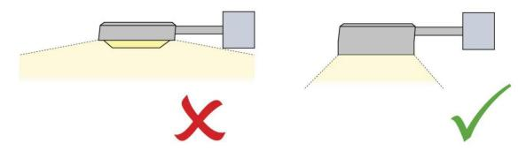
intensity (in candelas) at or above a vertical angle of 80° above nadir does not numerically exceed 10% of the luminous flux (in lumens) of the lamp or lamps in the luminaire.
